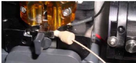
5. Cytometer>Cleaning Modes>Clean Flow Cell. When prompted, install a tube containing approximately 3mL of Windex. X2
