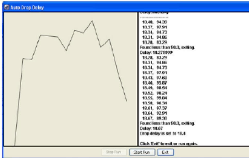
*Note: The drop delay value will remain fixed for subsequent sort experiments. It will not need to be adjusted again until the drop break off moves from the selected point aligned with on the Sort Layout window.*
