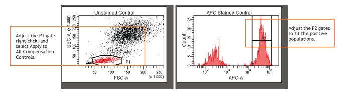
**10.** Select Experiment  $\rightarrow$  Compensation Setup  $\rightarrow$  Calculate Compensation  $\rightarrow$  Apply Only.
